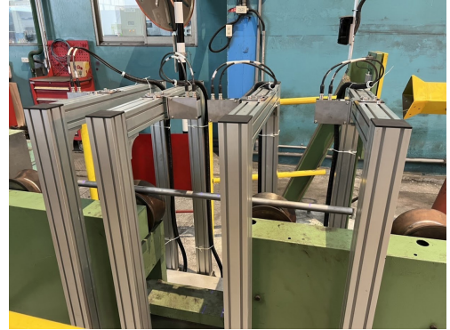
Fig.8. Segmental curvature measurement system constructed on the roller conveyor with the calibration bar.
